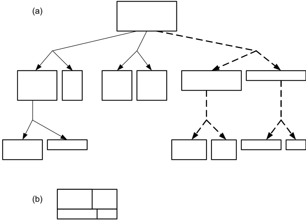
**Figure 2:** AND/OR-graph with a particular highlighted path (a) and the corresponding cutting pattern (b)
