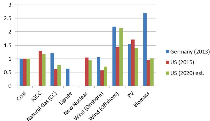
**Figure 5:** Levelized costs of electricity for different electricity sources. Index value, based on the electricity costs from coal in the respective study. Blue: costs in Germany 2013, determined by the Fraunhofer Institute for Solar Energy Systems (Kost et al., 2013); red: costs in the United States 2015, determined by the U.S. Energy Information Administration in 2015; green: costs in the United States 2020, estimated in by the U.S. Energy Information Administration in 2015.<sup>7</sup>
