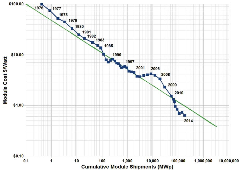
**Figure 7:** Solar panel module costs per Watt in dependence of cumulative module shipments. Source: wikipedia.de (data from ITRPV Edition 2015).
