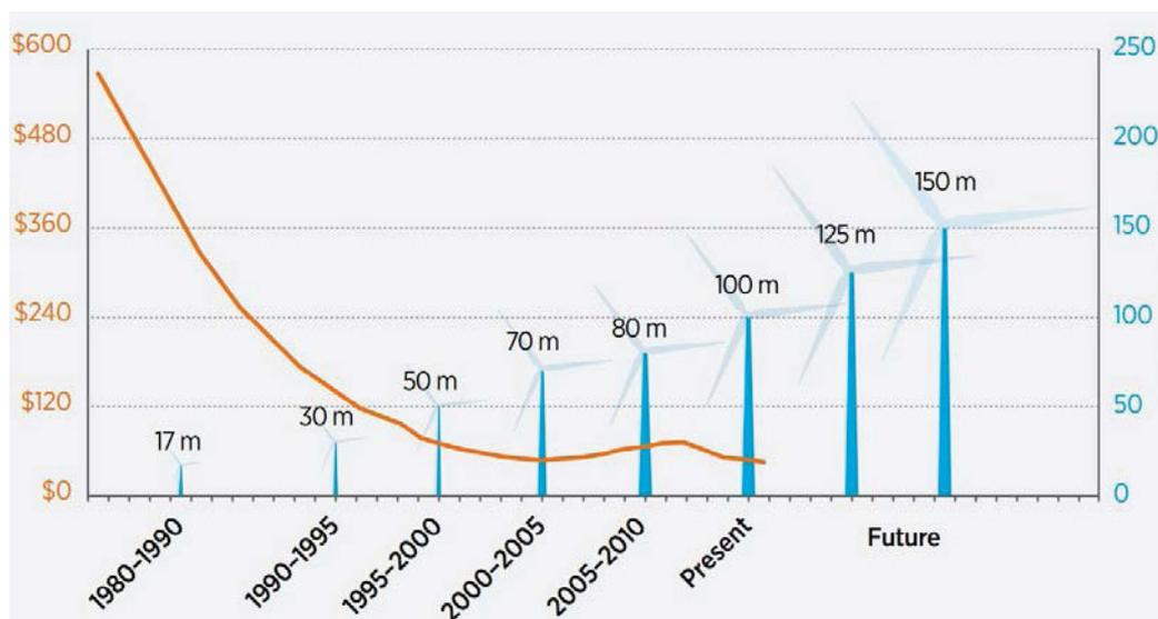
**Figure 7:** Development of levelized cost of energy for wind power (left) and height of wind power hubs (right). Source: US Department of Energy, DuVivier (2016).
