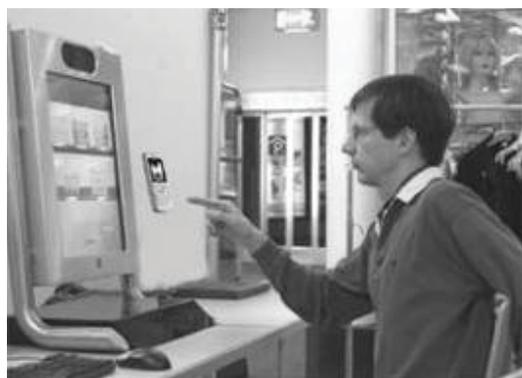
A camera based **hand tracker** detects hand gestures. It recognizes the position of the finger tip, which can be used for pointing at or for moving virtual objects represented with the stereoscopic display. The test person in front of the screen is able to touch, pick and turn the three-dimensional objects as if they were real
