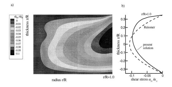
Figure 9: Shear Stress  $\sigma_{rz}/\sigma_0$  at the Instant of First Macrocrack Initiation a), Comparison to the Reissner Theory b)
