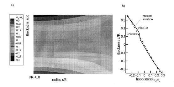
Figure 7: Hoop Stress  $\sigma_{\varphi}/\sigma_0$  at the Instant of First Macrocrack Initiation a), Comparison to the Reissner Theory b)
