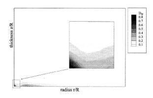
Figure 2: Hoop Damage $D_{\varphi}$  - Original Formulation by Murakami, Kawai and Rong
