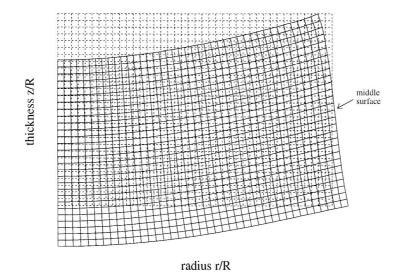
Figure 6: Deformation of the Plate under a Purely Mechanical Load p (Magnification  $\times$  1250)
