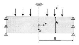
Figure 1: Simply Supported Plate Loaded by Constant Pressure p
