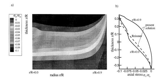
Figure 8: Axial Stress  $\sigma_z/\sigma_0$  at the Instant of First Macrocrack Initiation a), Comparison to the Reissner Theory b)
