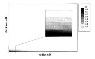
Figure 5: Radial Damage  $D_r$  - Modified Formulation
