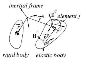
Figure 1. Multi Body System Consisting of Elastic and Rigid Bodies
