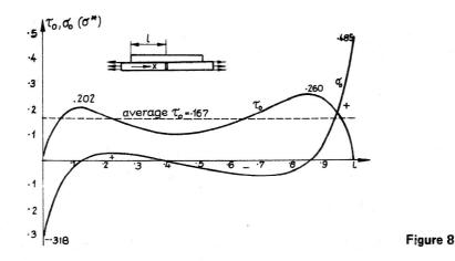
(2) The joint is made of pine cover plate and bars;  $E = 10^5 \text{ kg/cm}^2$ ,  $E_2 = .042 \times 10^5 \text{ kg/cm}^2$ ,  $G_1 = .075 \times 10^5 \text{ kg/cm}^2$ ,  $\mu_{12} = .238$ .  $h = 1.2h_1$ , h/l = 1/5.
