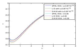
Figure 9. Horizontal displacement distribution vfor  $t = 0.05 \cdot 10^{-13}$ , t = 0.09.
