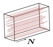
Figure 1: Visualization of the unidirectional long fiber CFRP. One-dimensional fibers are colored in red.
