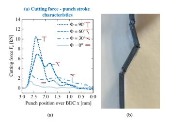
Figure 4: Experimental results: a) Cutting force over punch stroke (Shirobokov et al. (2015)), b) incomplete cut specimen after experiment.
