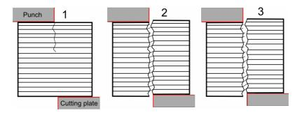
Figure 3: Visualization of the assumed process during shear cutting
