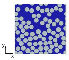
Figure 2: Exemplary geometry of the Repeating Unit Cell. Blue: matrix, gray: fibers.
