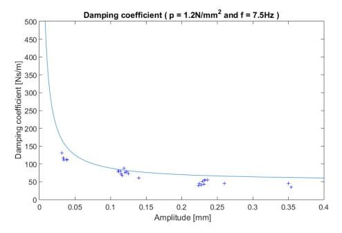
Figure 8: Damping coefficient for a surface pressure of  $1.2 \text{ N/mm}^2$  and an excitation frequency of 7.5 Hz
