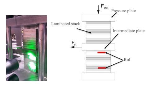
Figure 2: Principle of the measurement system
