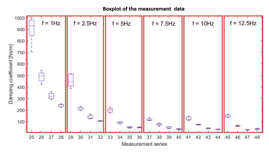
Figure 7: Boxplot of the measurement series with a surface pressure of  $1.2~\mathrm{N/mm}^2$
