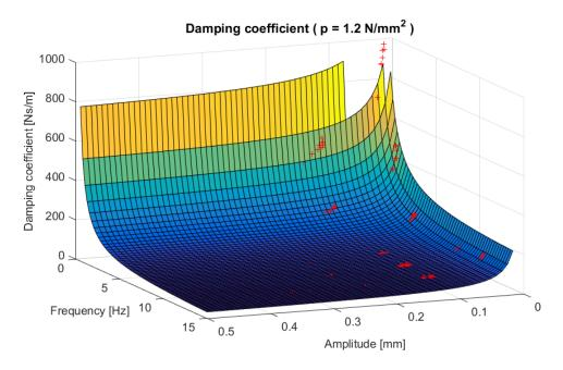
Figure 9: Damping coefficient for a surface pressure of 1.2N/mm<sup>2</sup>
