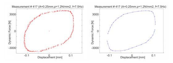
Figure 6: Hysteresis loop left: measurement data; right: linearized data
