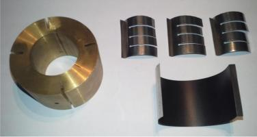
Figure 1. Parts of the foil bearing prepared for assembling
