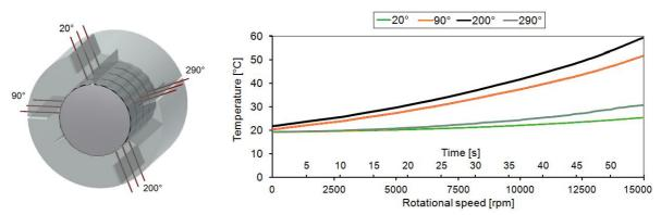
Figure 3. Thermocouples' location (left) and measured temperature of the central part of the foil bearing during acceleration of the rotor (right)
