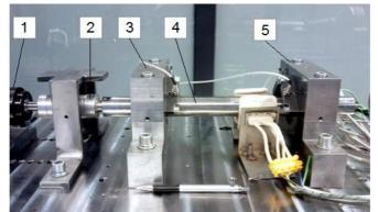
Figure 6. Configuration of the test rig for the rotor with two foil bearings (1 – electro-spindle, 2 – coupling, 3 – bearing support no. 1, 4 – shaft, 5 – bearing support no. 2)
