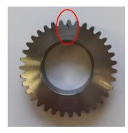
Figure 2: Artificially cracked planet tooth
