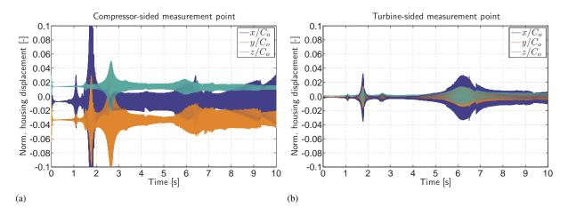
Figure 5: Normalized housing displacements for transient simulation of housing subsystem: (a) Compressor-sided measurement point. (b) Turbine-sided measurement point.
