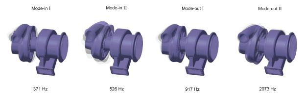
Figure 2: Modal analysis of housing structure which is rigidly clamped at the turbine inlet and outlet.
