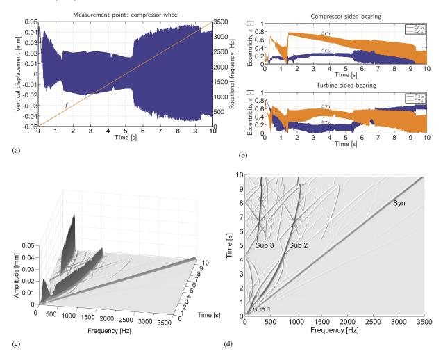
Figure 3: Run-up simulation of decoupled rotor bearing subsystem: (a) Vertical displacement of measurement point at compressor side (blue), rotational frequency f (red). (b) Compressor-sided inner/outer and turbine-sided inner/outer bearing eccentricities. (c)-(d) Waterfall diagrams (3D- and top-view) of plot (a).
