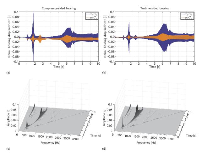
Figure 4: Transient simulation of decoupled housing subsystem: (a) Normalized housing displacement at compressor-sided bearing. (b) Normalized housing displacement at turbine-sided bearing. (c) Waterfall diagram of displacement in *x*-direction from plot (a). (d) Waterfall diagram of displacement in *x*-direction from plot (b).
