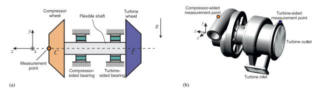
Figure 1: Mechancial model of subsystems: (a) Turbocharger rotor. (b) Housing structure.
