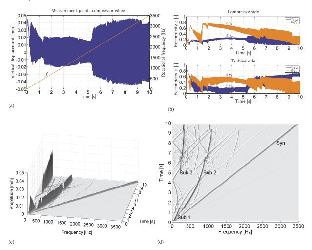
Figure 6: Run-up simulation of complete system (rotor subsystem): (a) Vertical displacement of measurement point at compressor side (blue), rotational frequency f (red). (b) Compressor-sided inner/outer and turbine-sided inner/outer bearing eccentricities. (c)-(d) Waterfall diagrams (3D- and top-view) of plot (a).
