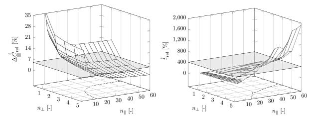
Figure 8. Relative norm of the stiffness difference (left) and relative computation time (right) for different combinations of element numbers per fibre in transversal and longitudinal direction. The transparent planes mark the acceptable values. The dashed lines belong to the mesh densities which correspond to these values.
