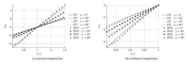
Figure 16. Comparison of material model's behaviour (Gauss point, GP) with data from a RVE containing 20% fibres. The material parameters are obtained from *Table* 10.
