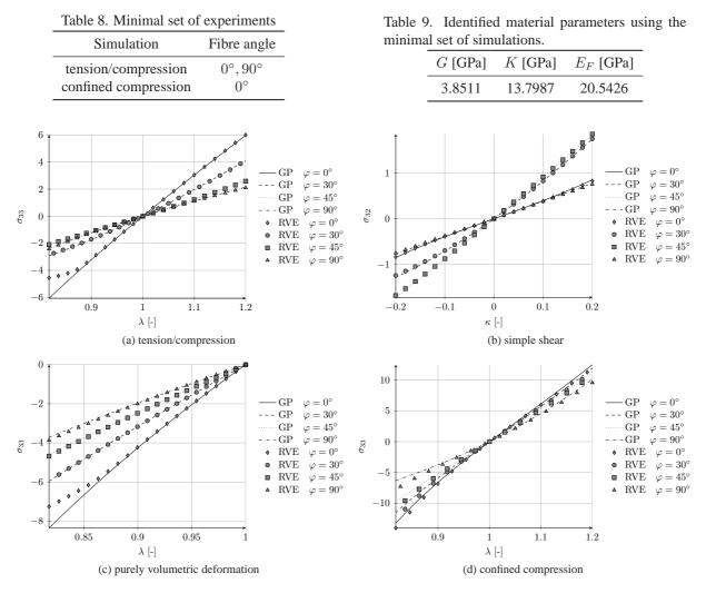
Figure 15. Comparison of material model's behaviour (Gauss point, GP) with data from the RVE (25% fibres). The material parameters are fitted to the minimal set of experiments.
