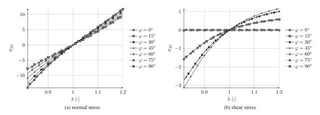
Figure 13. Cauchy stress over strain during purely volumetric deformation.
