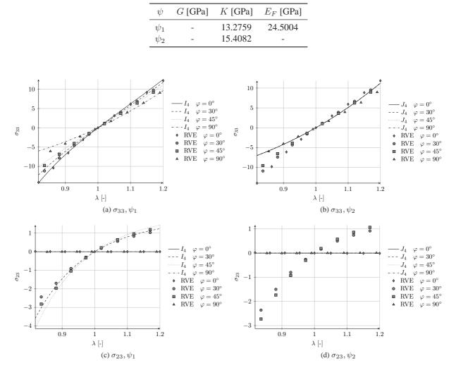
Figure 14. Comparison of material model's behaviour with data from the RVE (25% fibres) obtained during purely volumetric deformation. The diagrams show the longitudinal stress as well as the shear stress over the volume stretch for two different energy densities.
