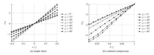
Figure 12. Cauchy stress over strain during simple shear (a) and confined compression (b).
