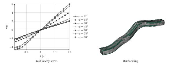
Figure 11. Cauchy stress over strain during tension/compression (a) and buckling of the RVE at values  $\lambda \leq 0.9$  (b).
