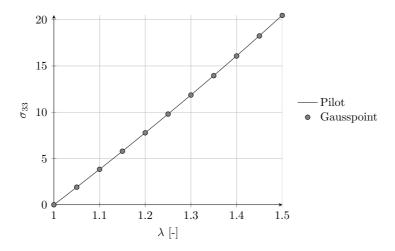
Figure 6. Verification of average stress obtained by evaluating the pilot's nodal forces. The results are compared to the stress values, which were received by averaging all Gauss points.
