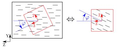
Figure 5. Left: Only the local coordinate system, and thus the applied deformation, is rotated in ABAQUS. The RVE and the fibres remain the same. Right: This is equivalent to deformations with rotated fibres.
