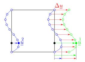
Figure 4. Principle of periodic boundary conditions. The displacements of the right edge  $(\underline{u}^1)$  are coupled to the displacements of the left edge  $(\underline{u}^2)$ . As an average and therefore constant displacement gradient is imposed on the entire surface, the displacement difference  $\Delta \underline{u}$  between right and left edge is constant for every pair of points.
