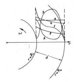
Fig. 3 Couette flow in a Searle-type rheometer
