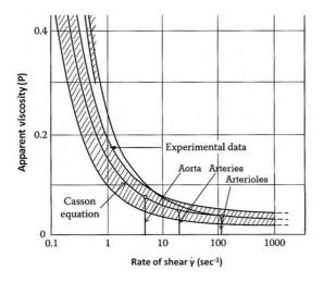
Fig. 4: Plot of apparent viscosity as function of shear rate (extract redrawn from (Whitmore, 1968) with permission)
