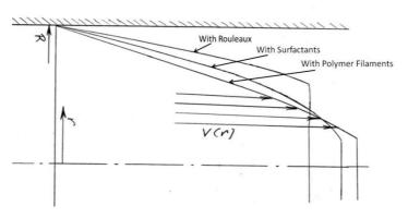
Fig. 8: Velocity profiles
