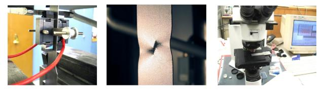
Figure 6. A specimen in the testing machine (*left*), deformation of the zone with artificial defects (*center*), measurement instrumentation (*right*)
