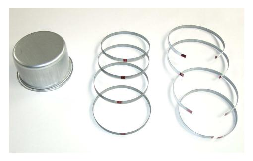
Figure 2: Springback experiment: cup, rings, open rings
