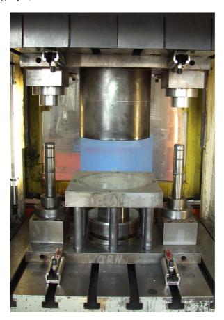
Figure 1: Cup drawing tool setup
