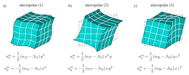
Figure 6: possible deformation modes reflecting micropolar deformation within the  $e_x/e_y$ -plane
