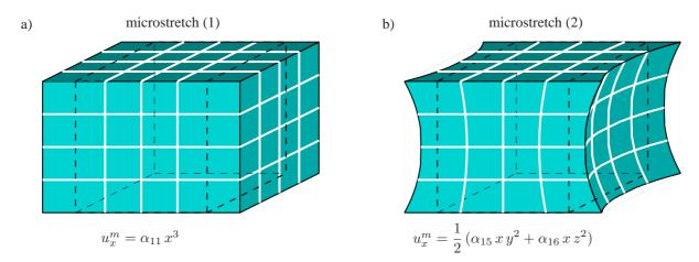
Figure 4: possible deformation modes reflecting microstretch into horizontal direction
