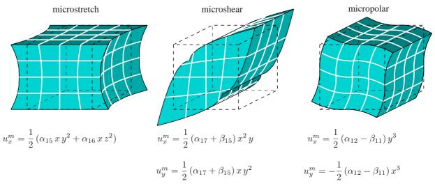
Figure 7: modes reflecting micromorphic extra deformation
