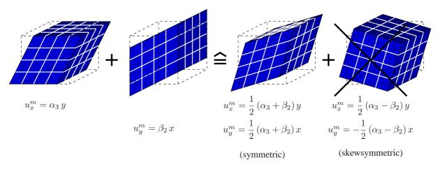
Figure 3: Split of shear mode into symmetric and skew symmetric part
