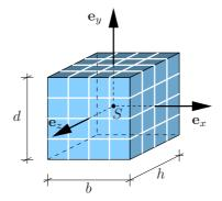
Figure 1: Cuboid TVE (dimensions b, d and h) and coordinate system
