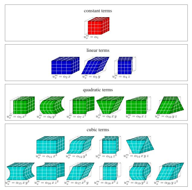
Figure 2: Deformation modes in  $e_x$ -direction up to terms of order three
