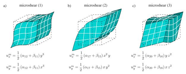
Figure 5: possible deformation modes reflecting microshear within the  $e_x/e_y$ -plane
