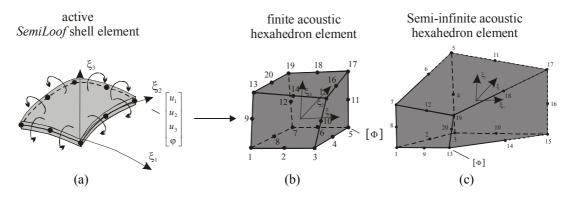
Figure 1. Coupling of shell elements and acoustic hexahedron elements: (a) piezoelectric *SemiLoof*-type shell element, (b) acoustic hexahedron element, (c) semi-infinite acoustic element
