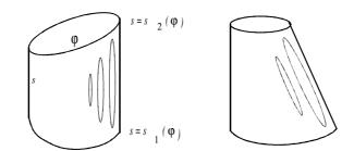
Figure 5: The localized vibration modes of cylindrical and conic shells
