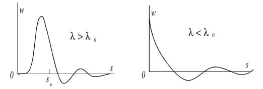
Figure 4: The vibration modes localized near the edge
