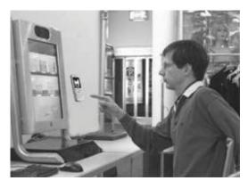
A camera based **hand tracker** detects hand gestures. It recognizes the position of the finger tip, which can be used for pointing at or for moving virtual objects represented with the stereoscopic display. The test person in front of the screen is able to touch, pick and turn the three-dimensional objects as if they were real
