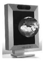
The Fraunhofer HHI **3D Kiosk system** offers simple intuitive handling as it presents any kind of object in a virtual manner on a large screen in photorealistic 3D quality (1600 by 1200 pixels; 21.3" screen). 3D-objects seem to float in front of the display for which no further technical additive like 3D-glasses or -helmet is necessary.
