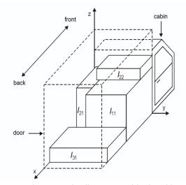
Figure 1: A loading space with placed boxes.
