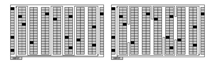
Figure 2.1: Example of S-Shape (left) and Largest Gap (right) heuristic in a single-block warehouse
