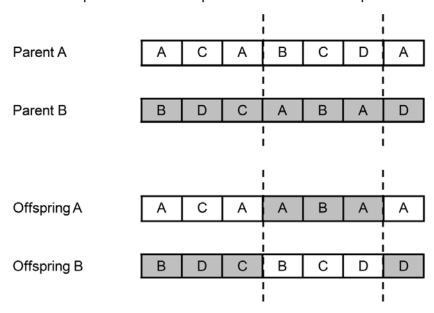
Fig. 4: Example of a two-point crossover
