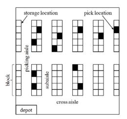
Fig. 1: Two-block layout
